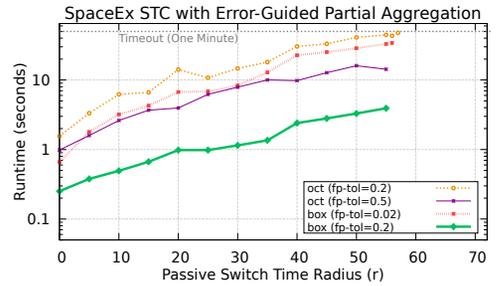
(b) SpaceEx with error-guided partial aggregation can analyze the system up to around  $r = 55$ .
