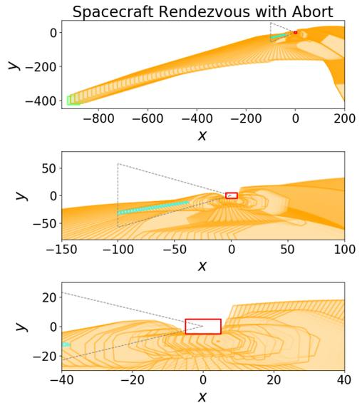
(b) The reachable set for the spacecraft rendezvous system at three different zoom levels is shown. Reachable states near the unsafe set (red square near origin) are deaggregated using the proposed approach until no unsafe states are reachable. A video of the computation is online at <https://www.youtube.com/watch?v=iXJlJnsxeN0>.
