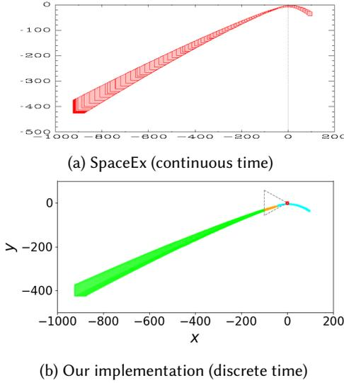
Fig. 5. The reachability plots using SpaceEx (top) in continuous time and our implementation based off Hylaa (bottom) in discrete time are qualitatively similar. The initial states are in the lower left of the plots, the unsafe states are near the origin. In this plot, the switch to the passive mode occurs at exactly time 140.
