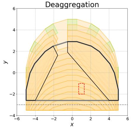
Fig. 1. The deaggregation process is shown for a two-mode system. Upon reaching an error mode (red dotted region), the fully aggregated set of states (gray large region), is split in half (two black regions), which no longer contain error states. A video of the complete computation is available online at <https://www.youtube.com/watch?v=SDzGKDBq5tM>.
