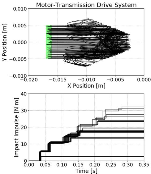
Fig. 10. One hundred random simulations are shown for the gearbox system on the x/y plane (top), as well as the total impact impulse over time (bottom). Notice the worst-case accumulated impact impulse, shown in Figure 11, was not observed in this simulation batch, demonstrating that simulations can miss important system behaviors. A video of the simulations is online at <https://youtu.be/IBwKe2g4Rb0>.
