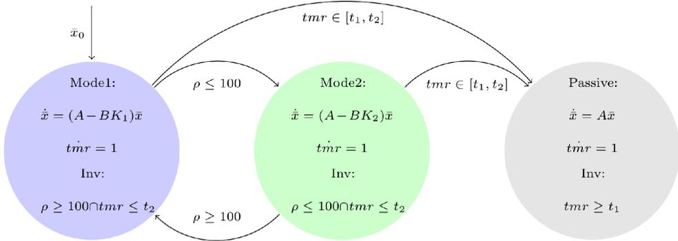
Fig. 4. Hybrid automaton model for our case study (image from [8], which also include the dynamics matrices). We check for passive safety from time  $t_1 = 70 - r$  to  $t_2 = 70 + r$ , where  $r$  is a model parameter.
