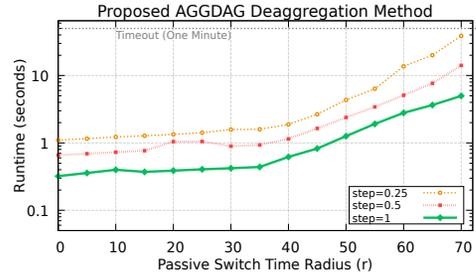
(a) The proposed AGGDAG approach can analyze up to the full  $r = 70$ , even for the smallest time step.
