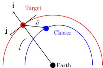
Fig. 3. Collisions are checked between spacecraft in orbit in relative coordinates (image from [8]).
